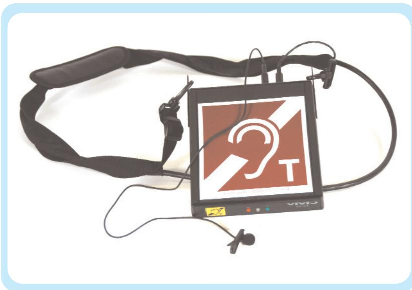
In busy or noisy environments, hearing aids amplify both background noise and the spoken word. Hearing induction loops employ a microphone to pick up the spoken word which is transmitted to a hearing aid set to T mode by the wearer, greatly improving access to goods and services for customers with a hearing impairment.
